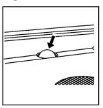
The light sensor for the DRL and AUTO headlamp feature is located on top of the instrument panel. If the sensor is covered, it will prevent it from sensing light, and the exterior lamps may come on whenever the ignition is on.
